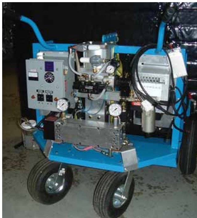
Heated Predator III Spray Rig's unique design allows for easy maneuverability on the job and output of 2 gallons/min.
